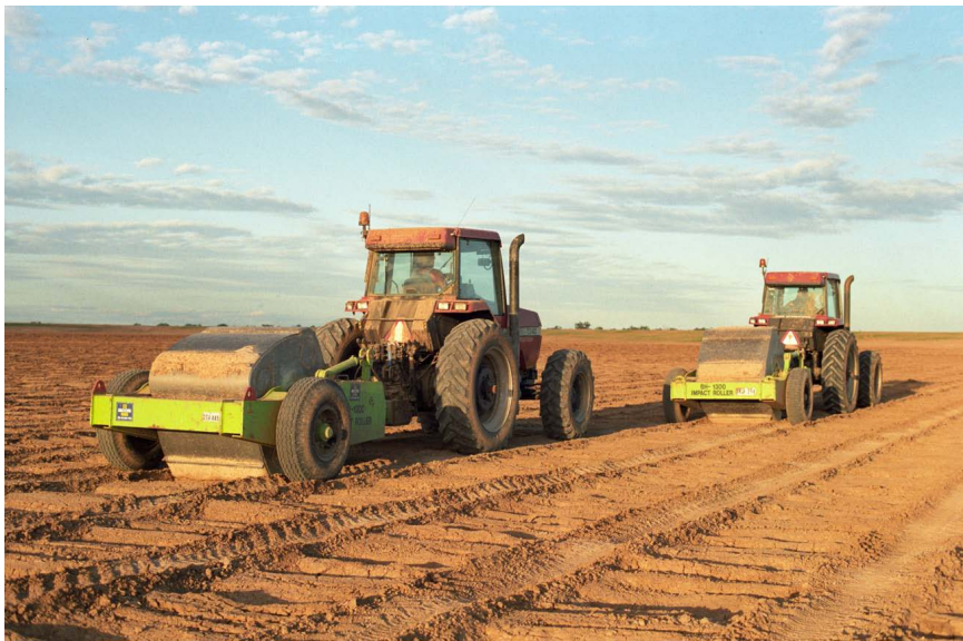
Figure 1.6.16 – An example of an impact roller at work (photo courtesy of Broons)
