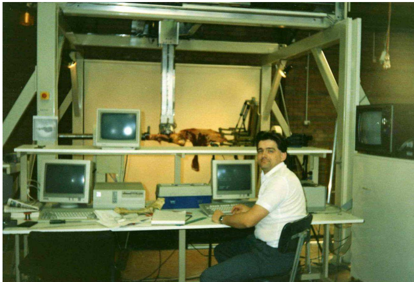
1989 7 axis force feedback robot for deboning beef
